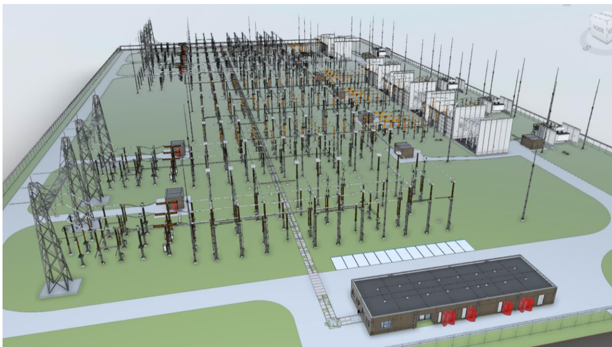
Figuur 2: 3D-model 380kV station
